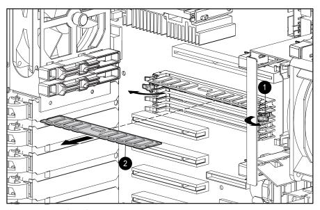
Figure 2-28. Removing a SDRAM DIMM
